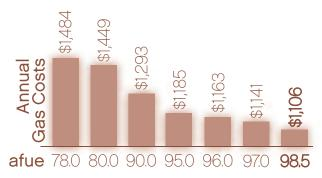
The Carrier® Infinity® 98 is the most efficient gas furnace that you can buy.\* This gas furnace offers plenty of potential for annual savings with outstanding gas efficiency. Compared to today's minimum efficiency models, the Infinity 98 can deliver estimated savings of about \$343 annually on your gas costs.† If you are replacing an older furnace, you can save even more. Variable-speed blower and inducer motors contribute electrical savings as well to complete the utility savings story.
